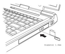
Figure 4-4 Manual release with the eject hole
